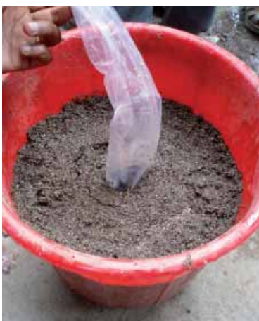
Collapse of the 'borehole' (bucket)
