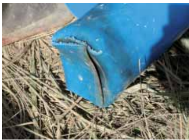
Bottom end closed by cutting and bending
