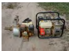
Motor pump set (1) 3,5-4,5 Hp engine, 2" pump outlet (able to pump 15-20 m 3 /h)
